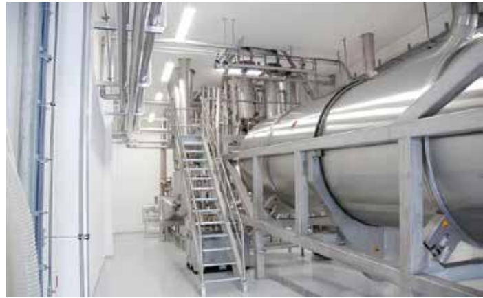
Bühler Cerex puffing system: view of the Expansion Channel
